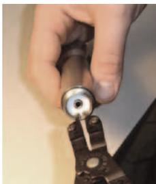
3. Once the snap-ring has been removed, press gently on the white disk to force one end up for easy removal.
