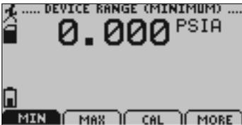
*Displays values indicating minimum pressure detectable by the DL12.*
