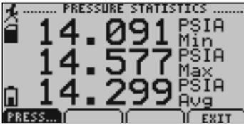
*Displays statistics (maximum recorded value, minimum recorded value, and average recorded value) for the pressure channel.*
