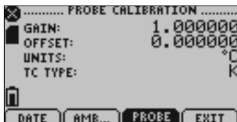
*Displays calibration information for external probe channel.*
