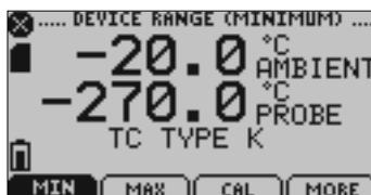
Displays values indicating minimum internal temperature and external probe data (for thermocouple selected) detectable by the DLI-T.
