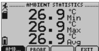
Displays statistics (maximum recorded value, minimum recorded value, and average recorded value) based on channel (Internal Temperature or External Probe).
