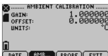
*Displays calibration information for internal temperature channel.*
