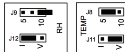
Figure 2: Jumper settings for display units. CO 2 is set for a 4 to 20 mA and to 10V output, humidity is set for a 4 to 20 mA output, temperature is set to 0 to 5V output. (NOTE: Jumper names)
