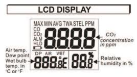
CO<sub>2</sub> measurement is shown in top display
