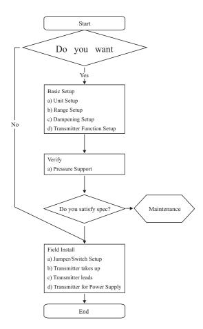
[Figure 4-1 Installation Flow Chart]
