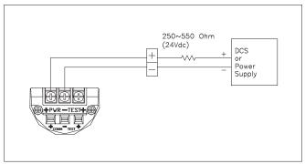
Figure 4-2 Wiring the 3100 Pressure Transmitter
