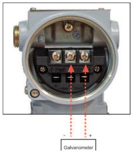
Figure 4-3 Picture of Transmitter Wiring Terminal
