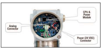
Figure 6-3 Structure of Electronics Module
