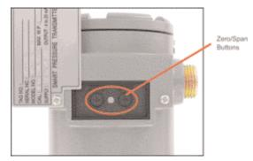
Figure 3-4 Transmitter Zero/Span Configuration Buttons
