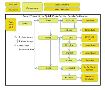
[Menu Tree for Zero+Span Button Function]
