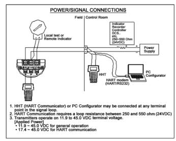
[Figure 3-5 Connecting the Transmitter to HHT]
