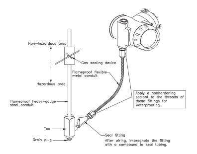
Figure 4-4b Typical Wiring using Explosion-Proof Conduit
