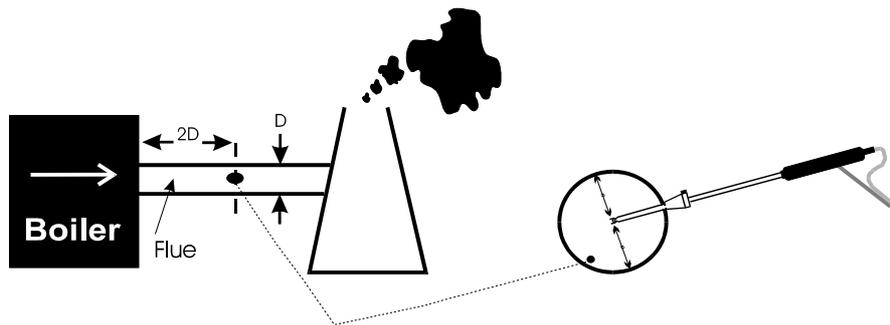
Use the probe's depth stop cone to fix it in flue diameters from  $\frac{1}{4}$  to  $\frac{4}{5}$  inch, 6 to 21 mm. Its maximum operating temperature is 1112°F / 600°C.
