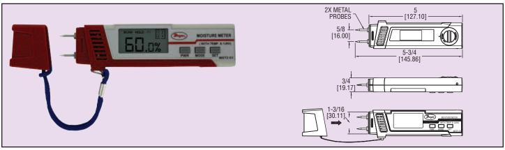
The Model MST2-01 Digital Moisture Meter is a high-accuracy instrument used for determining the moisture content in wood, bamboo, and other various materials. This unit also has the ability to measure ambient temperature and relative humidity. The large digital LCD makes measurements easy to read, while the hold function makes them easy to record. The MST2-01 includes a protective cap, two replacement pins, and one battery.
