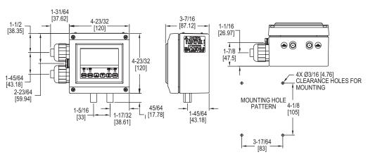
The SERIES DHII takes all the features of the standard Digihelic® Pressure Controller and packages them in a robust NEMA 4 (IP66) housing.
