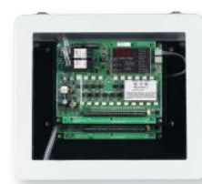
Master board stacked with channel expander
