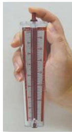
For high scale reading, finger covers hole
